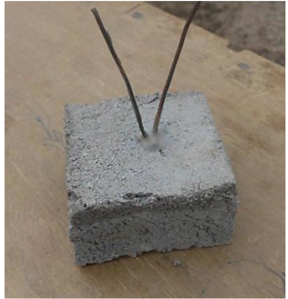
Concrete spacer to be used in all RC works.
