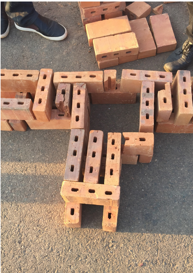
Dry stack of a RLB wall sample
